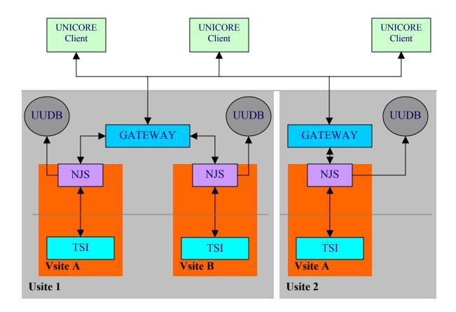
Figure 3: UNICORE Deployment Example
